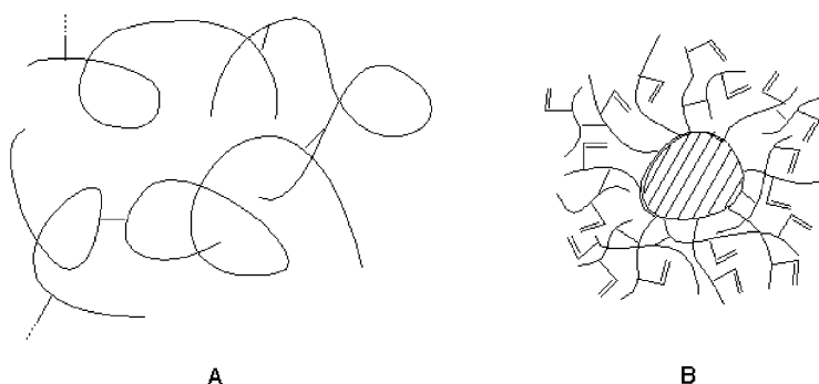
Figure 2. Two extreme structures of crosslinked polymers as (A) an ideal network polymer and (B) a microgel.
